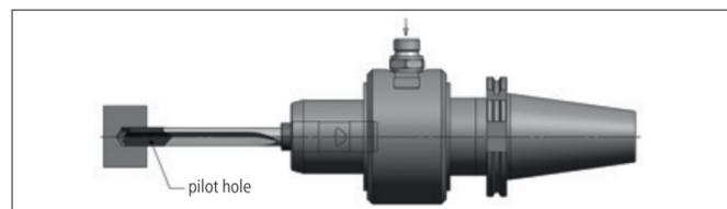
The gundrill is a single-edged tool without self centering. When positioning the drill, the tool must be guided through a drill bush or a pilot hole.
