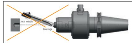
Using botek gundrills other than directed may cause personal injury. Tool breakage and unsupported gundrills can be extremely dangerous. Please use with caution and care.
