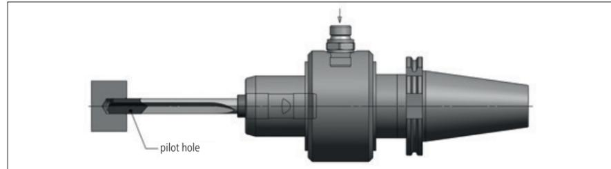
4. Tools support: unsupported drill length should never exceed the dimensions as shown on table (previous page). If the unsupported drill length is exceeded the drill might cause injury. Do not exceed 40 times diameter unsupported!
